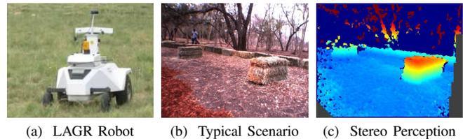
Fig. 1: The LAGR robot (left); sample image from an outdoor scene (center); stereo obtained from onboard cameras (right).
